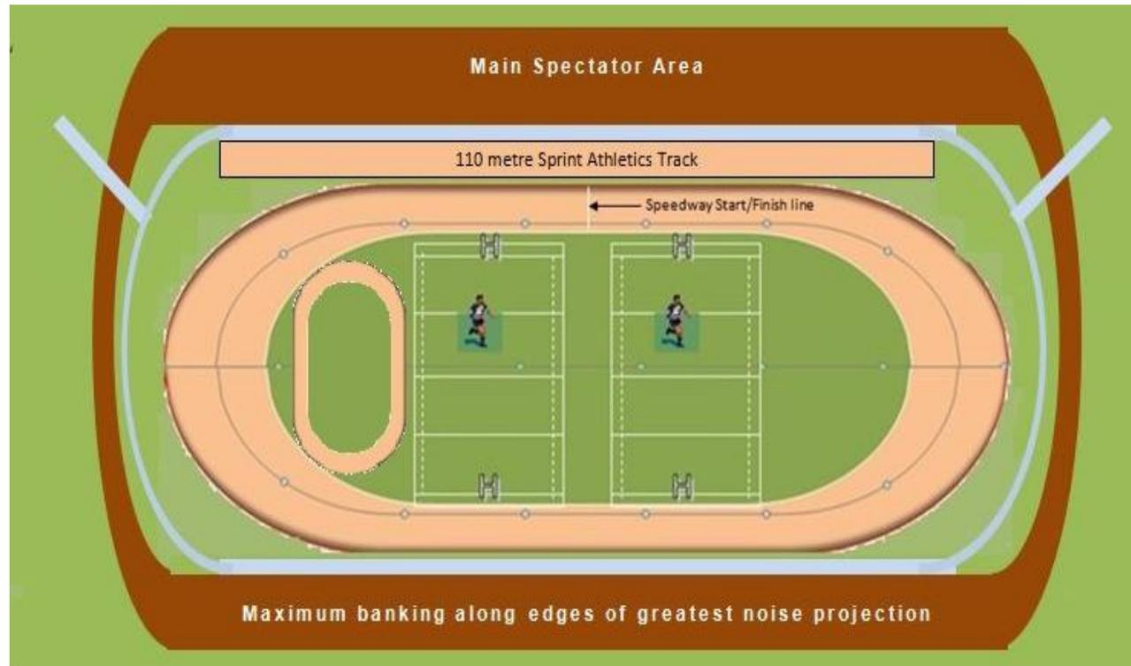
Drainage can be a problem for granite-based tracks, and can lead to event cancellation on the grounds of rider safety. Tracks are often raised half a metre or so, and encircled by spoon drains (in blue) wherever necessary, and a means by which excess water can leave the stadium. While modern speedway machines leave only rubber particles on the track surface, some mechanism will be required to ensure that nothing reaches natural water courses.
